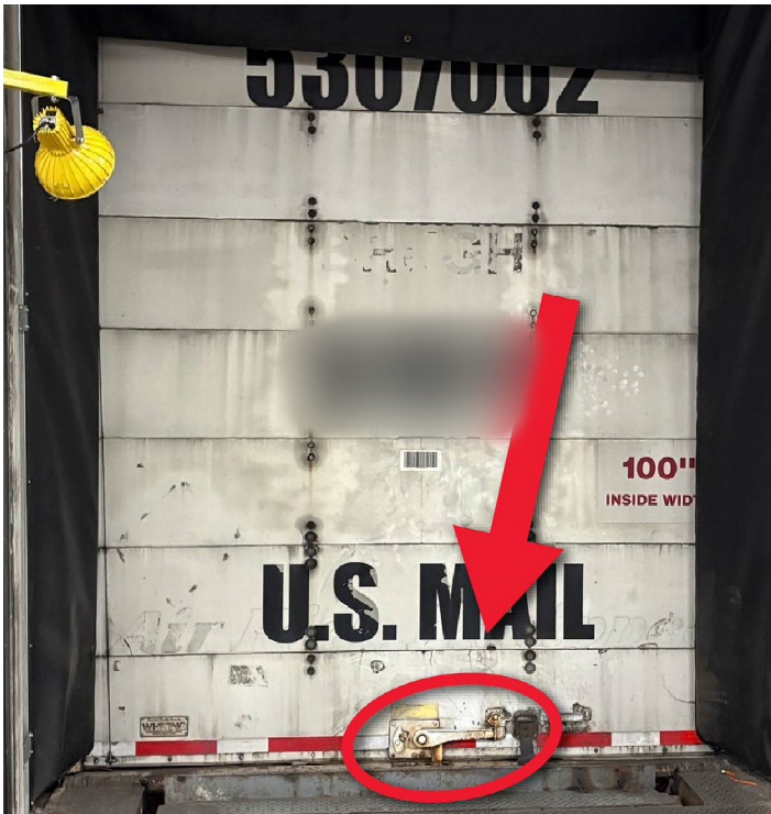
Figure 4. Unsecured Trailer Door
