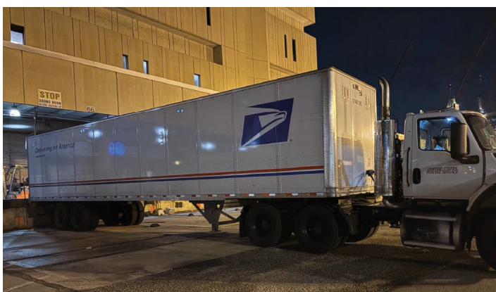
Figure 5. Examples of Trucks and Trailers Without Wheel Chocks
