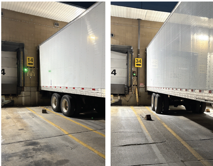
Figure 2. Examples of Truck and Trailer Without Wheel Chocks
