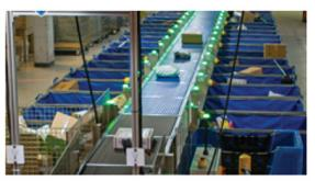
The ADUS automates the sorting of smaller packages (up to 30 pounds). ADUS machines can sort 2,600 packages per hour to the carrier level for delivery. In comparison, the hourly target distribution rate for a clerk to manually sort packages is 270 per hour.
