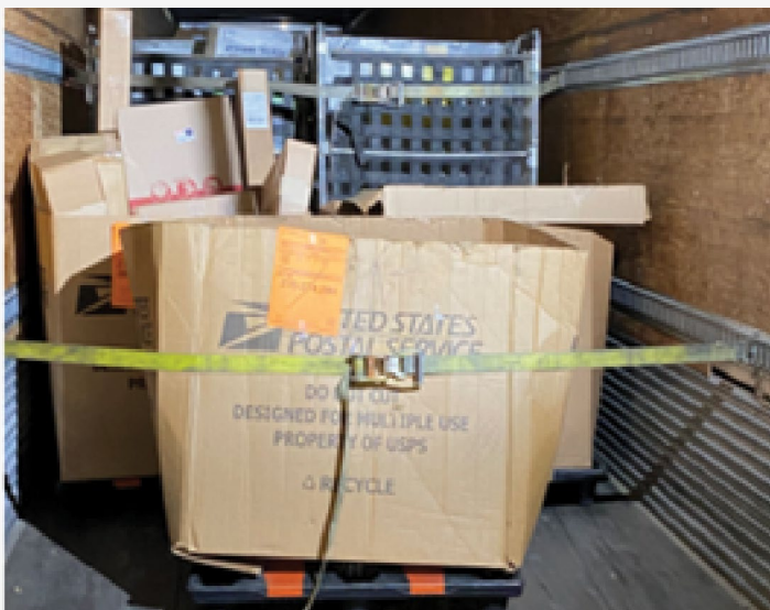
Figure 1. Trailers With Improperly Placed Straps
