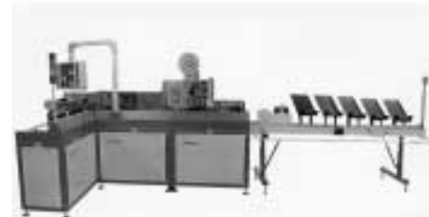
The OIG found the Postal Service underutilized 30 of 83 tabbing systems. The tabbing system allows open-ended mail such as fliers and brochures to be handled by high-speed automation equipment.
