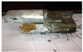
Figure 2. LLV starter damaged by salt water
