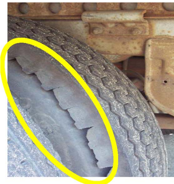
The shredded tire cap on this leased trailer is an out of service deficiency.
