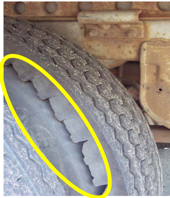
(Above) The shredded tire cap on this leased trailer is an out of service deficiency. Photograph taken at New Jersey International Bulk Mail Center May 1, 2002.
