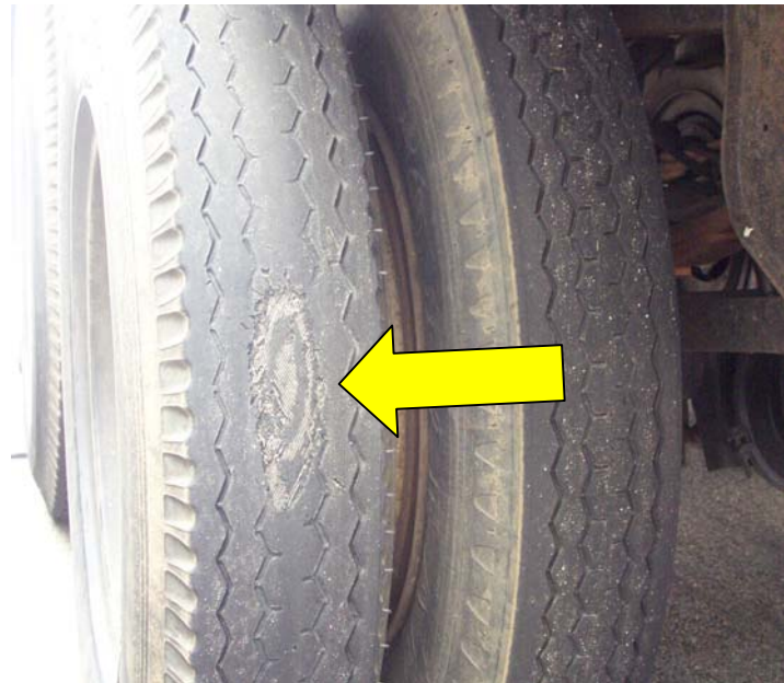
The worn tire on this leased trailer is an out of service deficiency. Photograph taken at New Jersey International Bulk Mail Center May 1, 2002.
