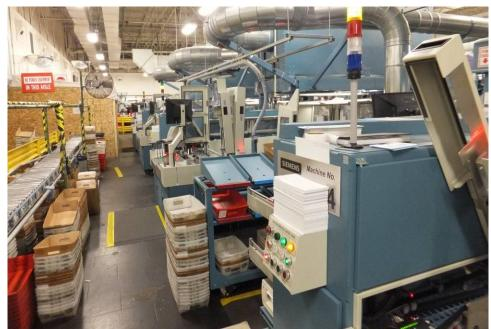
Source: OIG photograph, dated June 26, 2012. Cancelled letter mail from the Automated Facer Canceller System is trayed and placed on the rollers, where they must then be loaded on rolling stock and moved to the next operation.
