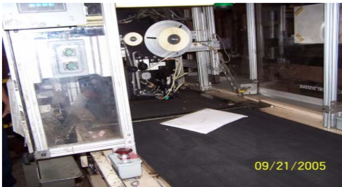
Illustration 3. Barcode printer applicator that had a missing label roll cover. Barcode labels were misapplied or were applied skewed, and sometimes missed the package entirely. (Jacksonville BMC, September 21, 2005)
