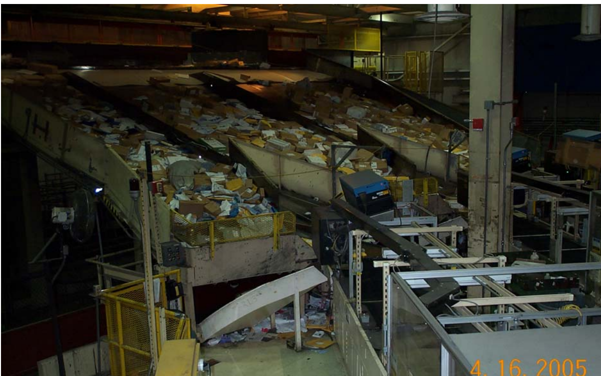
Illustration 2. View of primary sorting operation at the Washington BMC with backlog of parcels not being worked. Introduction of the OCR would allow some primary mail to be processed on the secondary sorters, thus relieving congestion and reducing dependence on the primary operation. (Washington BMC, April 16, 2005)
