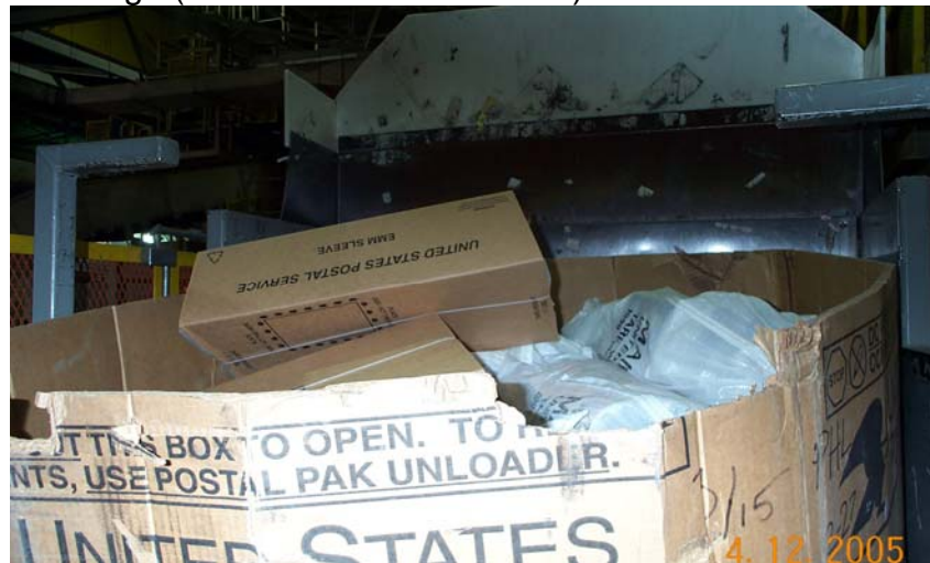
Illustration 4. Trays dumped onto the sack sorter machine broke open, resulting in loose mail (April 12, 2005, 10:34 a.m.).
