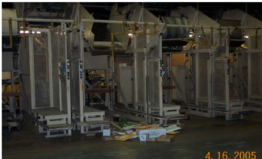
Illustration 7. Parcel sorter machine mail allowed to drop on floor. This mail had to be manually loaded into mail containers. (April 16, 2005, 10:30 p.m.)
