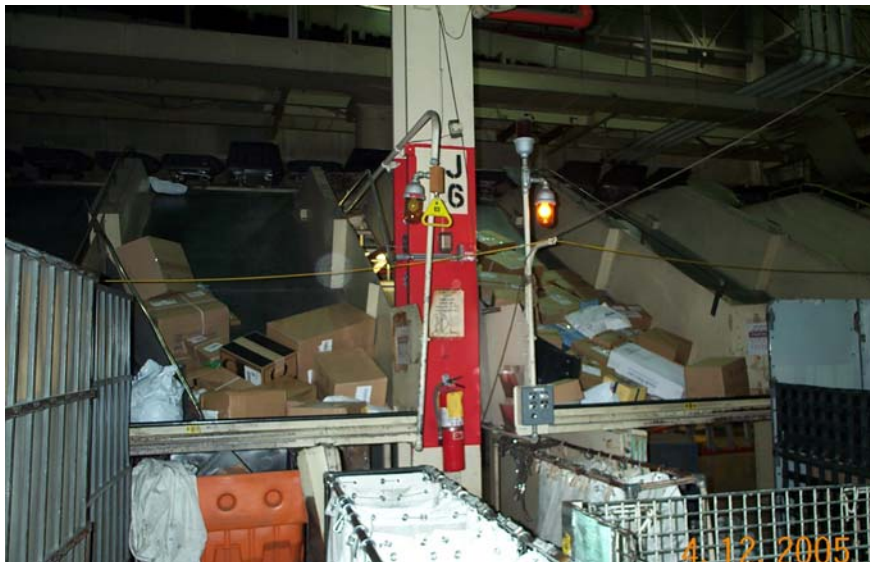
Illustration 6. Parcel sorter machine discharge slides were not cleared promptly, resulting in a high reject rate and poor productivity. (April 12, 2005, 2:00 a.m.)
