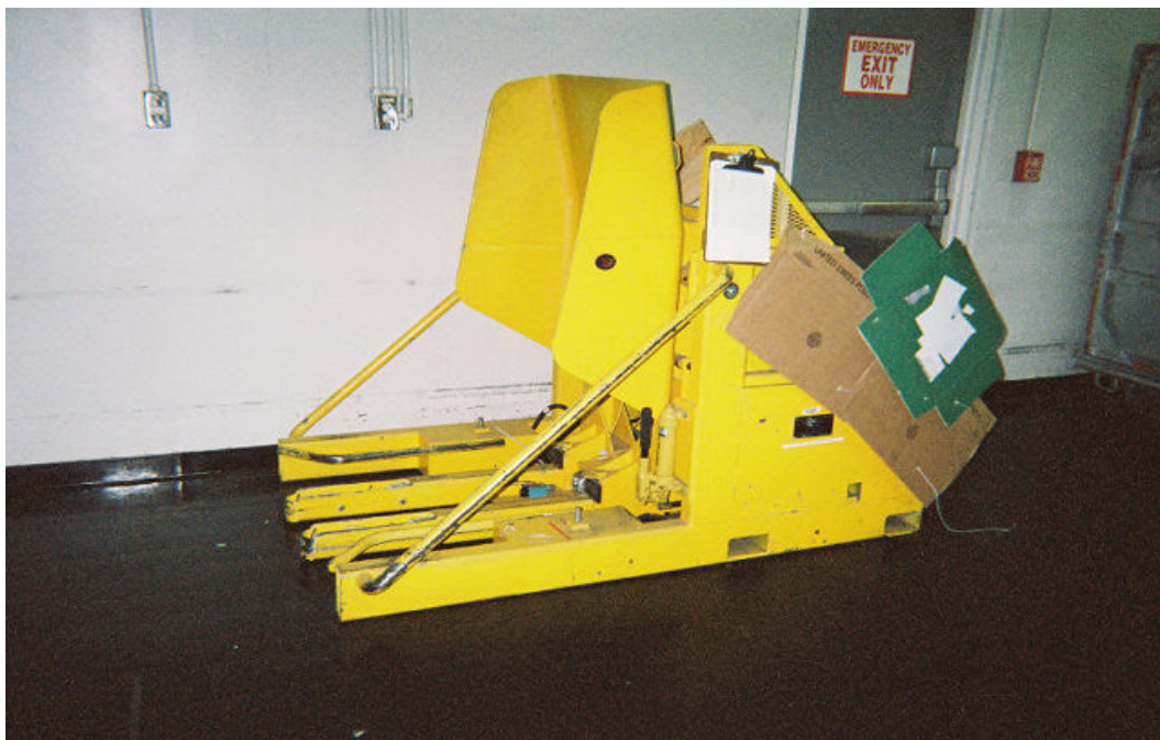
Illustration 4. The current hamper dumper in the Customs Unit was seldom used because mail normally arrived in over-the-road and all-purpose containers. The hamper dumper cannot take mail from these types of containers and dump it onto a conveyor belt to begin processing.
