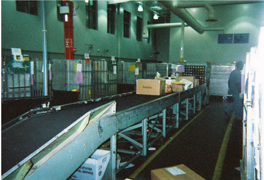
Illustration 3. Manual sorting of parcels. A Linear Integrated Parcel Sorter would streamline this process.
