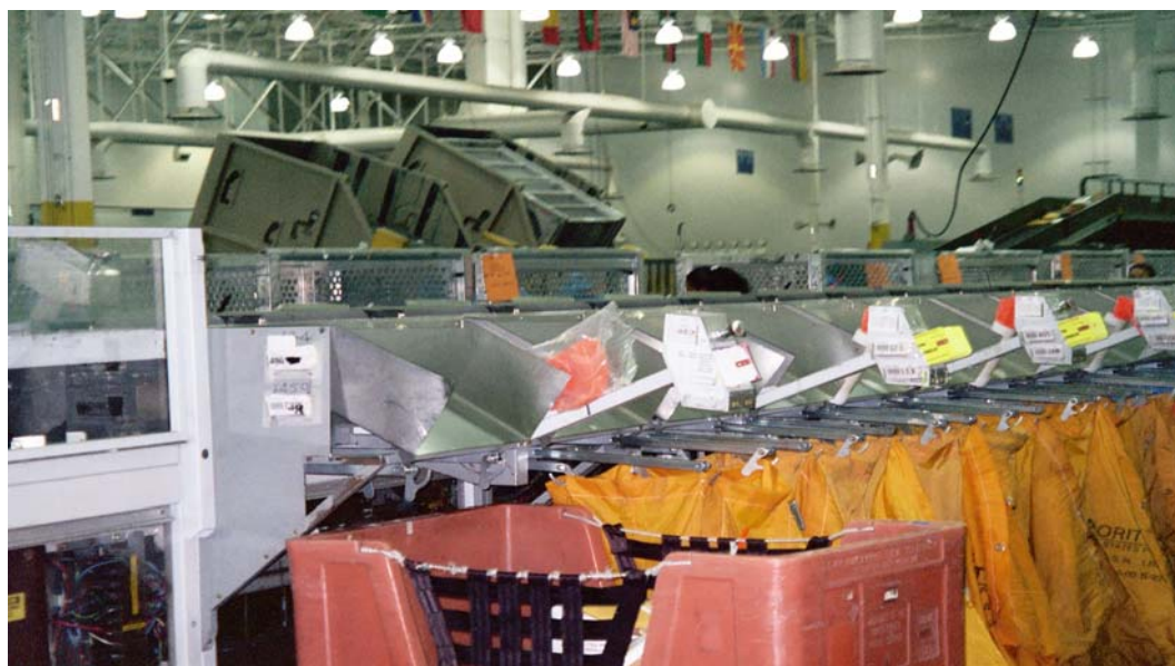
Illustration 6. After the operators key parcels (see Illustration 7), the parcels move down a conveyor belt and fall into separation bins based on ZIP Codes. 10 Parcels that are addressed to ZIP Codes that do not have individual bin separations fall into the red hamper. As seen above, the red hamper is half full and will need to be replaced soon. Additional employees will be needed to pull bins that fill up quickly and manually process mail where individual bins do not exist. An extension to the SPBS would provide additional separation bins and allow this mail to be worked more efficiently.
