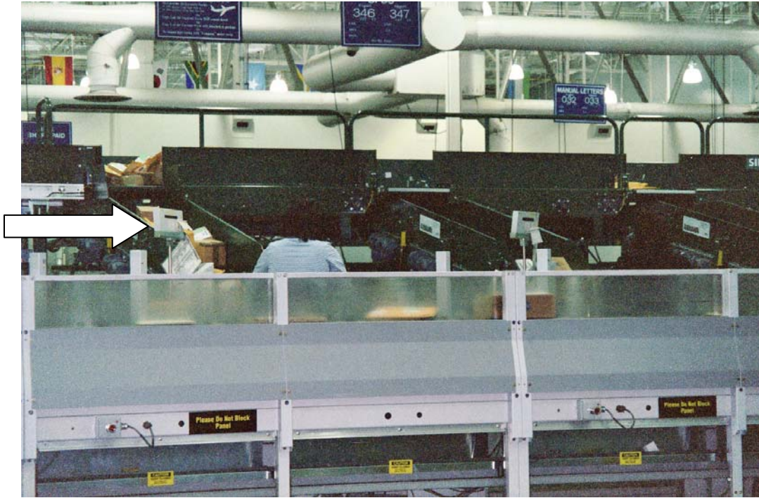
Illustration 7. This picture shows an operator keying parcels on the SPBS. (See Illustration 6.)
