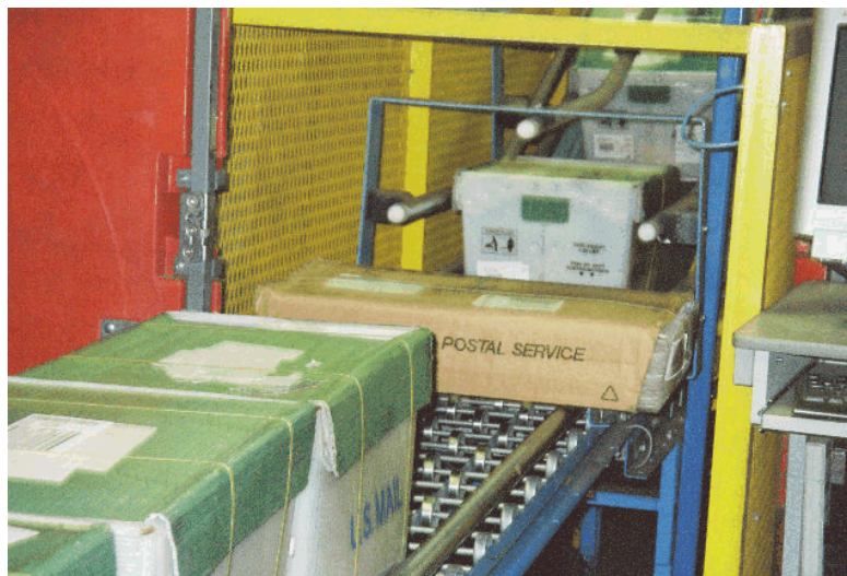
Illustration 7. Inbound tray line with a letter tray jammed into rollers, stopping the conveyor and backing up mail bins. (April 2004, New York ISC.)
