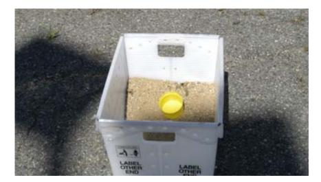
Plastic mail container with absorbent material used to catch leaking oil.
