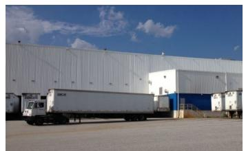
Figure 2. Spotter Truck Moving Trailer in the Atlanta NDC Yard
