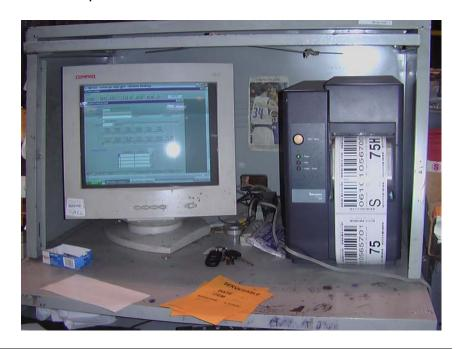
After quality clerks inspect pallets and authorize payment for work completed, they use the MTESS to print an inspection placard and attach the placard to the shrink-wrapped pallet.
