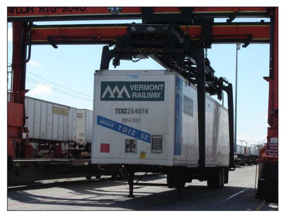
Highway trailer being lifted onto rail flat-car for rail transportation. Burlington Northern Santa Fe Rail Yard, Los Angeles, California, April 28, 2005.
