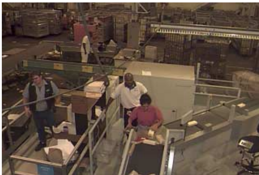
OIG Representative Observes Postal Service Employee Input Test Barcode Data During Successful Y2K Test of a 'Small Parcel and Bundle Sorter'
