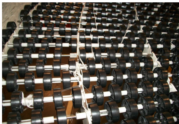
Figure 1. String from Broken Bundles Entangled in APPS Machine
