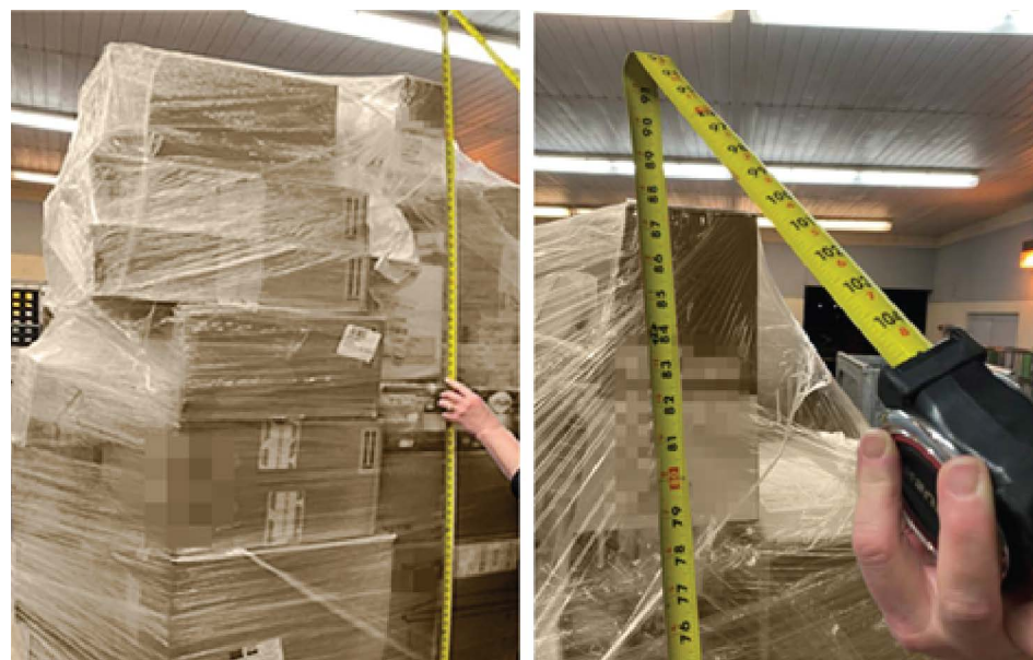
Figure 1. Pallet Exceeding Maximum Height Requirement
