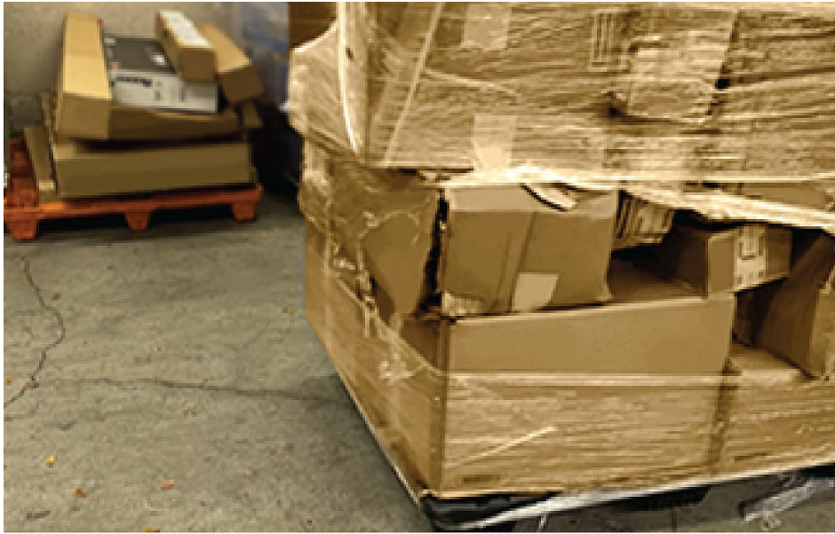
Figure 2. Heavy Packages on Top of Pallet – Crushed Packages Underneath
