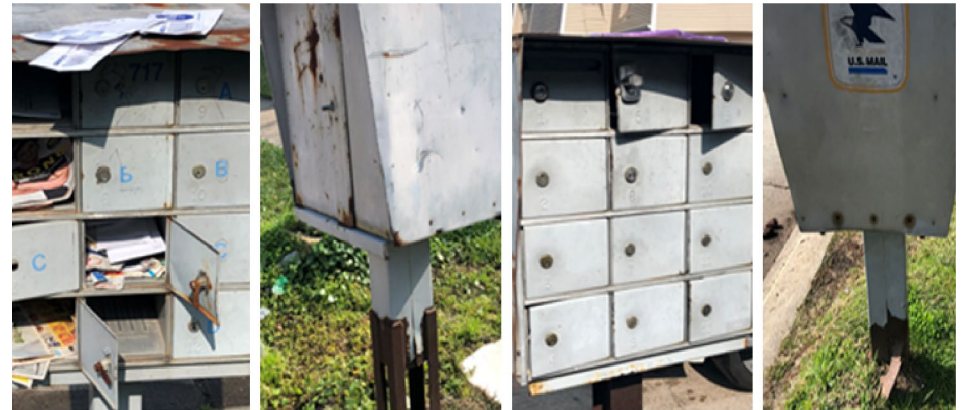
Figure 7. Damaged Cluster Box Units
