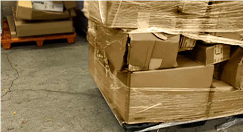
Figure 3. Heavy Packages on Top of Pallet - Crushed Packages Underneath
