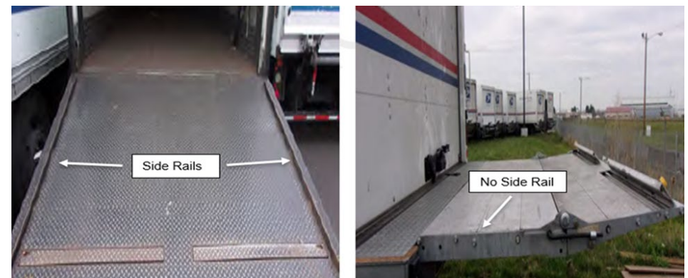
Figure 4. Side Rails on Lift Gates
