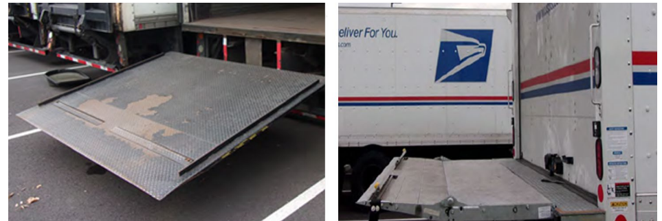
Figure 6. Comparison of Size of Prior Lift and New Tuck Under Lift Gate
