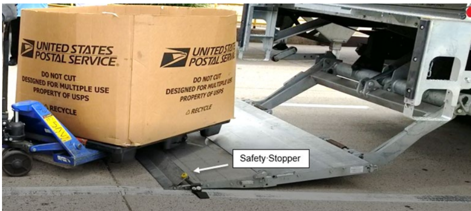
Figure 9. Pallet Jack With MTE Getting Stuck
